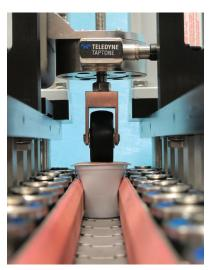
Single size pod samples (coffee) being tested in T550 C-LP w/TDLC.
